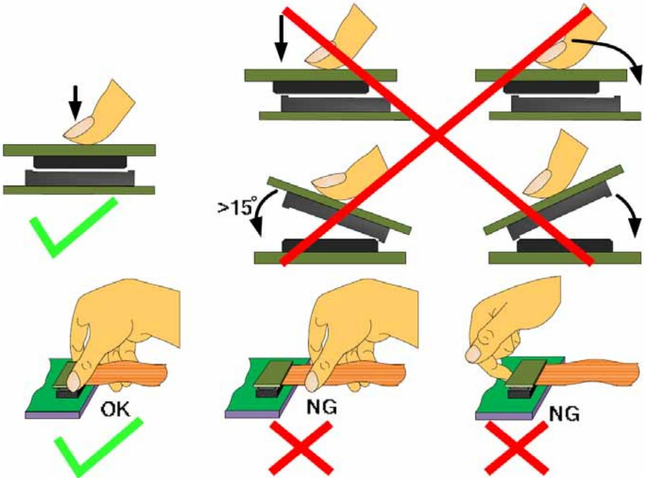
**Precaution for assemble the module with ZIF connector:**
